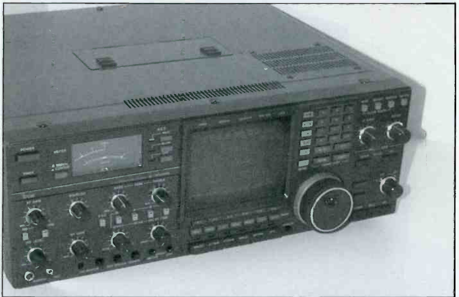
The large CRT display in the center is the most prominent feature on the R-9000 receiver. The CRT clearly shows the current use of the multi-function buttons below. All other controls are widely spaced and easy to operate. This radio is equally at home in the HF bands or as a VHF/UHF communications receiver.
