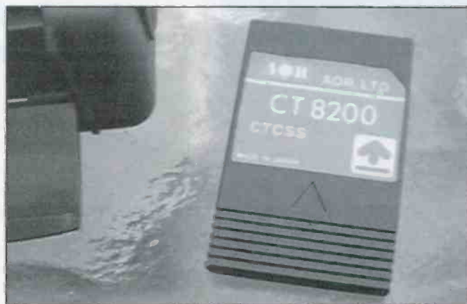
One of the most exciting and promising features of the AR-8200 is the ability to add features with plug-in cards. Several cards are already available to add features such as CTCSS, memory storage, and audio recording.
