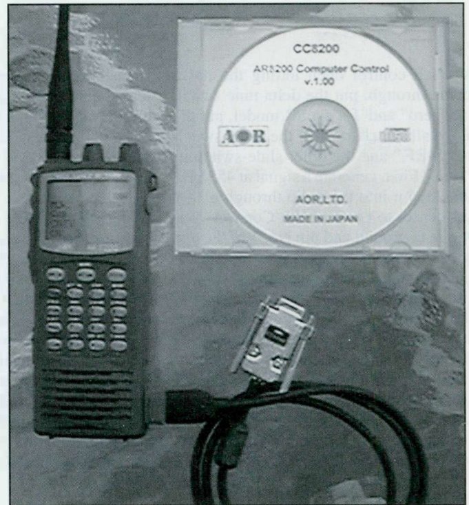
The AR-8200 is a completely redesigned unit. Notice the computer connection on the side panel. The AOR Computer Connection kit (CC-8200) includes the cable and software for your Windows-based computer.
